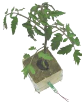
Fig. 2 Real-time measurement of conductivity in the tomato seedling experiment.
