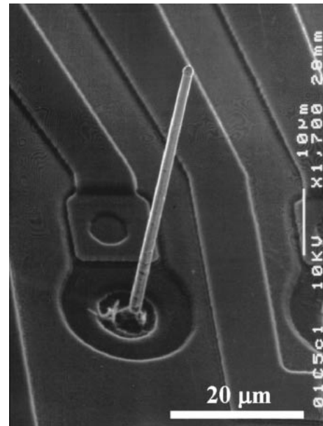
Fig. 5. SEM image of a Si microprobe 60\mu\text{m} in length and 2\mu\text{m} in diameter VLS-grown at 3 \times 10^{-3}\text{Pa} , at 600^\circ\text{C} for 2 h. Note that the predetermined length of the VLS Si probe can be realized by changing the growth time.
